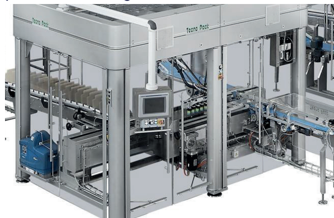
TECNO PACK TRAY FILLING SYSTEM for jaffa cakes, biscuits and sandwich biscuits placed on the edge
